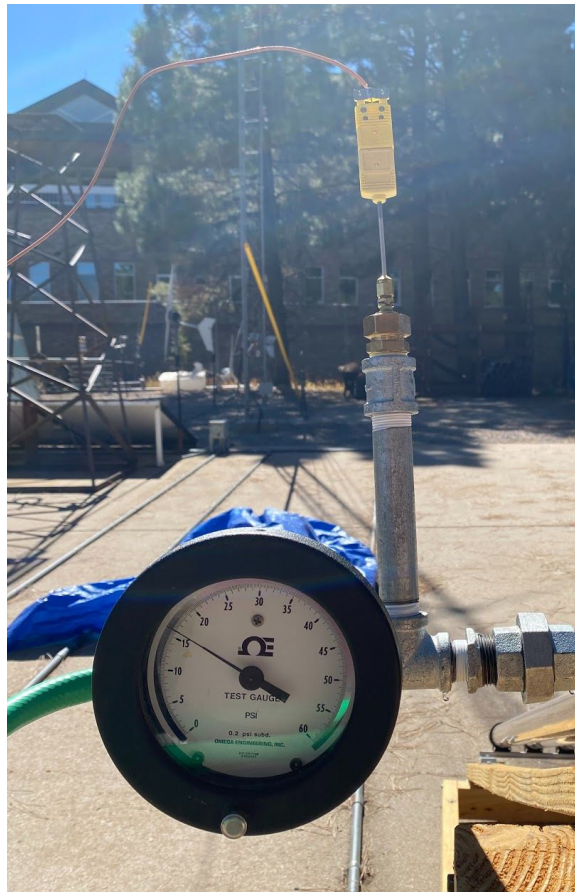
Figure 14. Thermocouple and Pressure Gauge at inlet of panel
