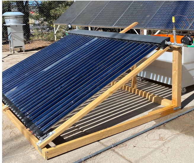
Figure 12. Full testing system with hydraulic bench and panel frame
